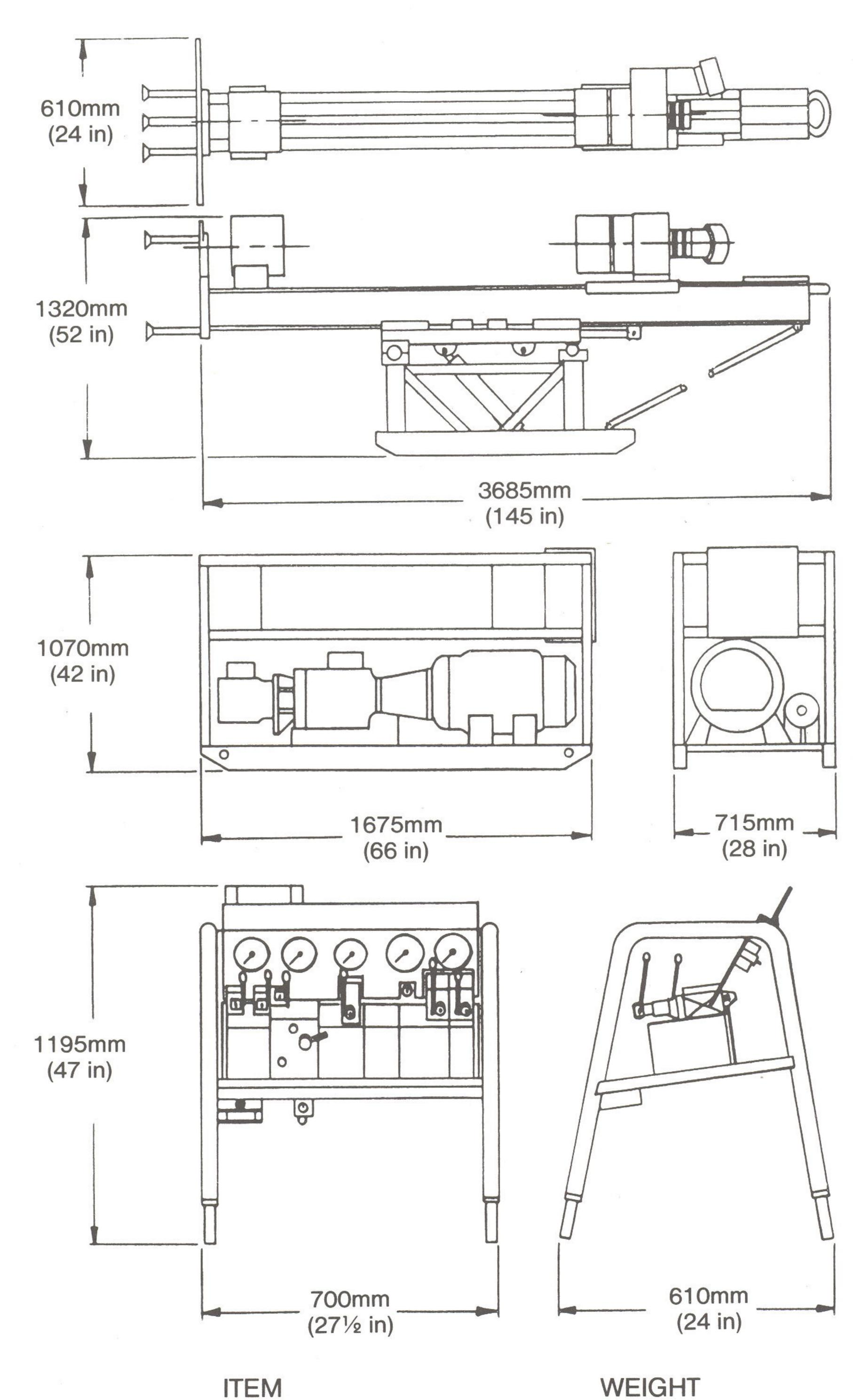
DRILL FEED FRAME ASSEMBLY (INCL. SKID)
